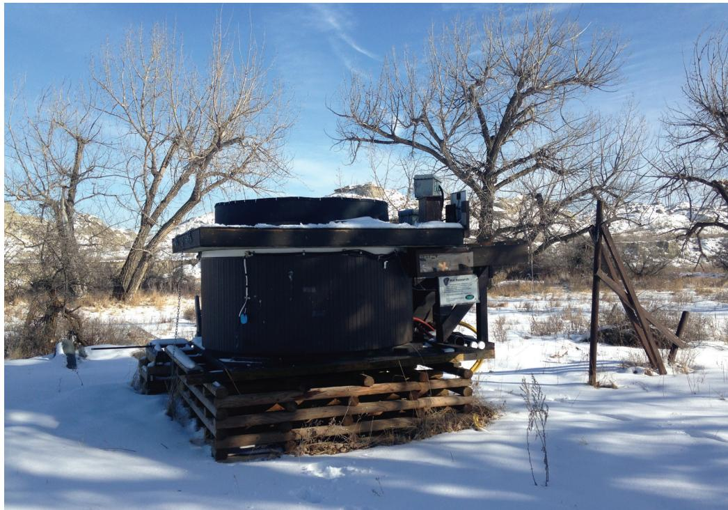
FIG. 1. Photograph of the 1,700 l heated water tank installed in Dinosaur Provincial Park from 2008–2015 as a continuously accessible source of water all winter. Tank water was enriched with deuterium ( $^2\text{H}$ ) to levels of +400–925‰
