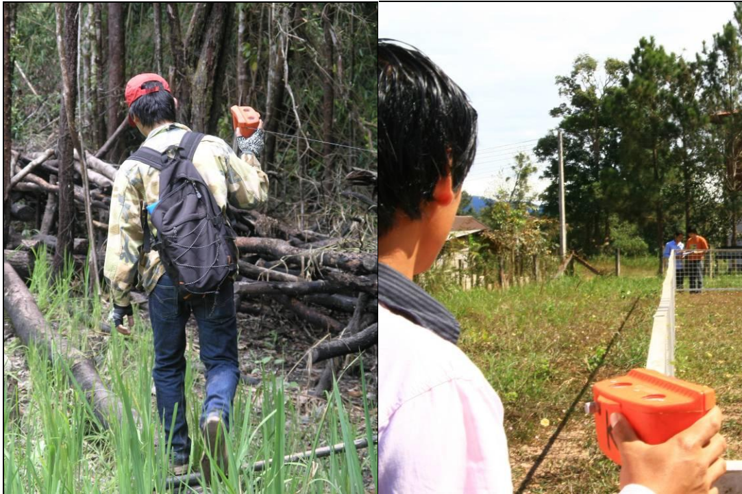
Figure 17. HEC monitoring team members use a hipchain to measure a distance between two points.
